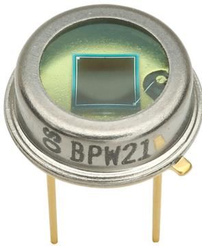
FIGURE 1 – Photodiode
