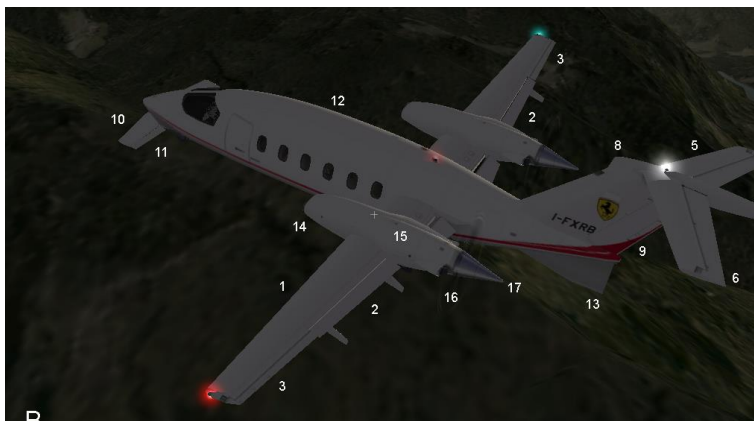
3-Surface aircraft, Mid-tapered wing, Twin-pusher engine Retractable-tricycle landing gear
