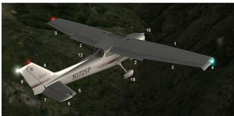
Conventional, High-tapered wing, Single-tractor engine Fixed-tricycle landing gear
