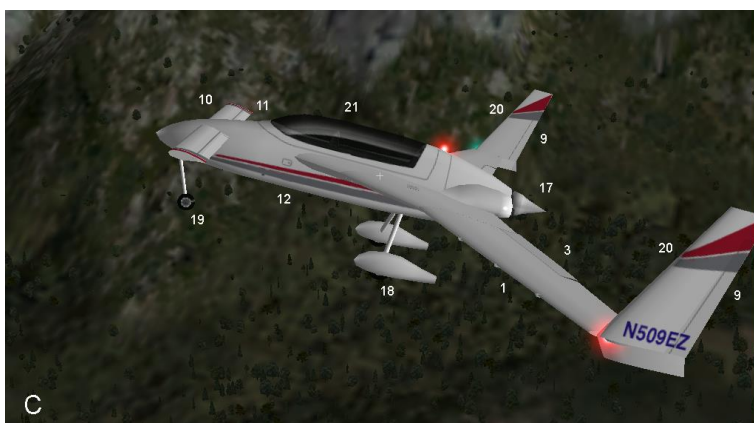
Canard aircraft, Mid-tapered-swept wing, Single-pusher engine, Fixed-tricycle landing gear
