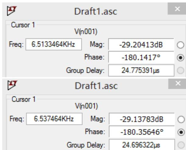
$$\left| \left. \frac{d\varphi}{d\frac{\omega}{\omega_0}} \right|_{\omega=\omega_0} \right| = \left| \frac{\omega_0}{2\pi} \frac{d\varphi}{df} \right| = \left| \frac{\omega_0}{2\pi} \frac{(-180,1417 + 180,35646) / 180 \times \pi}{6513,3464 - 6537,464} \right| = 1,0098$$
