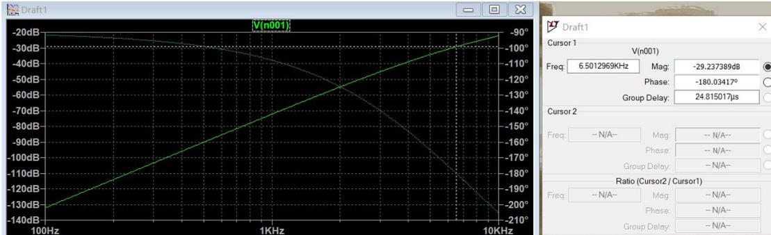
En  $-180.03^\circ$ ,  $f_0=6501.30\text{Hz}$ ,  $A=-29.24$
