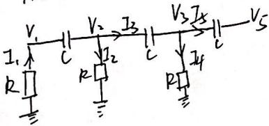
$$I_1 = \frac{0 - V_1}{R} = j\omega C (V_1 - V_2) \Rightarrow V_2 = \left(1 + \frac{1}{j\omega R}\right) V_1$$
