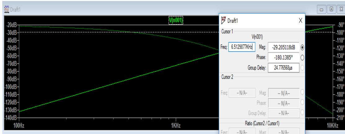
On calcule la fréquence  $f_0 = \frac{1}{2\pi\sqrt{6}RC} \approx 6497.5\text{Hz}$ ,  $A = \frac{1}{\|\beta(j\omega_0)\|} = 29$
